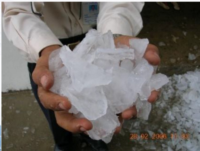
Pic. 1 – Hard, dry ice from water defrost ice harvester
